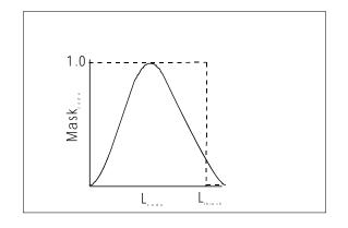
Figure 6: Generation of mask signal from luminance image
