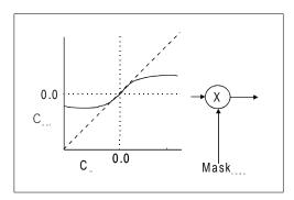
Figure 5: Modification of chrominance signal by the mask signal
